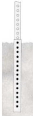
Figure 3 - Telescoping Steel Sign Support
